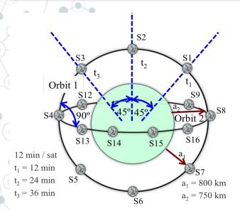
S2 and S3 connect each other inter-satellite link by an because the distance them short between is assuring low energy consumption.
