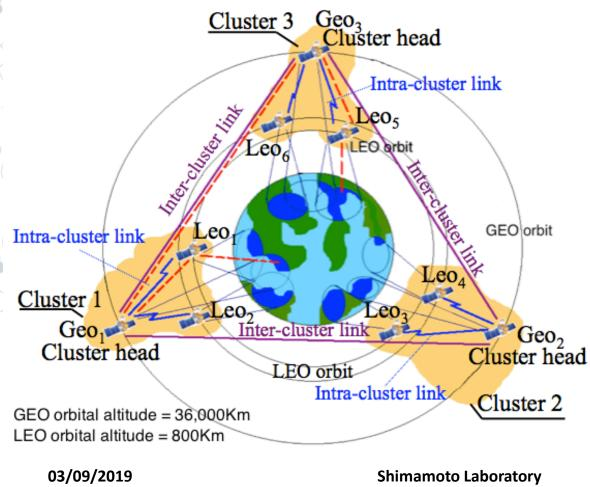
The proposed system consists of three satellite clusters sharing tasks by intra-cluster and intercluster links.
